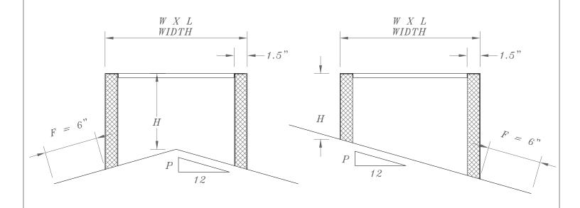
$\begin{array}{cccc} W & = & WIDTH \\ L & = & LENGTH \\ H (MINIMUM) & = & 6" (152.4MM) \\ \end{array}$
